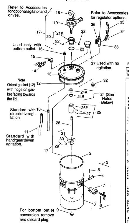
Open side of Shaft Seal (24A) faces downward.
